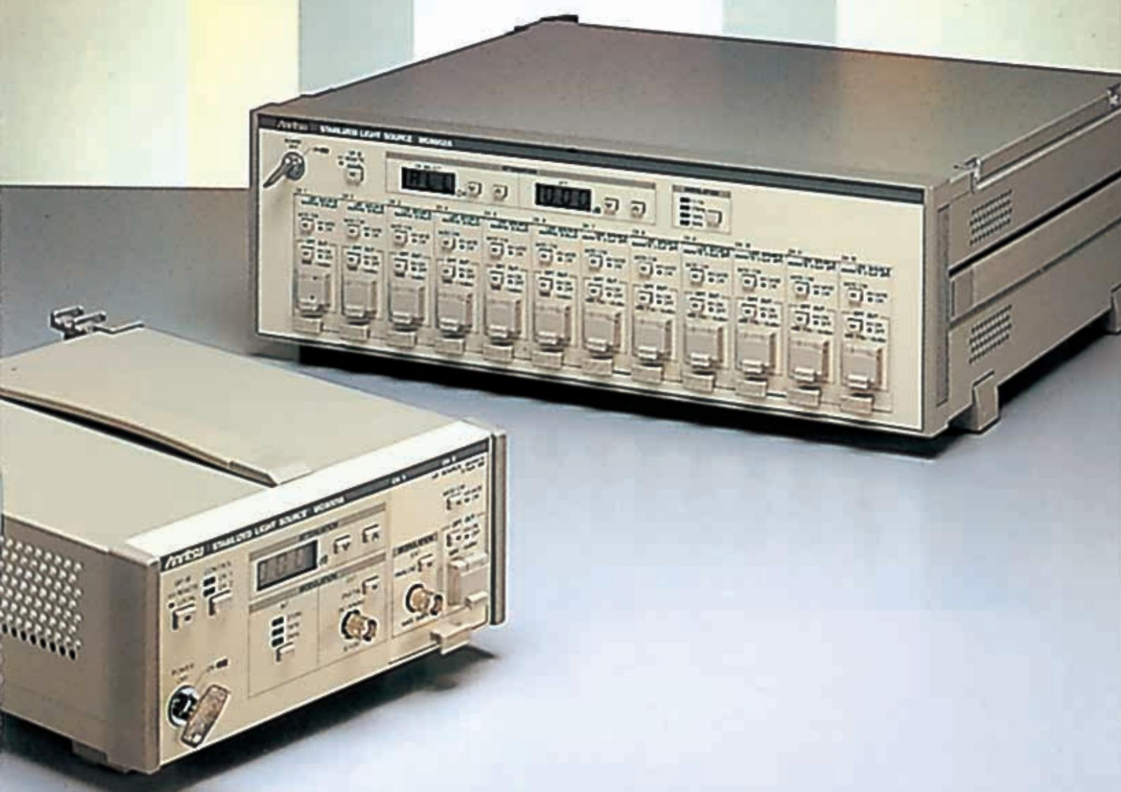
The MG9001A/MG9002A can be used as stabilized light sources for different applications by changing the light source units. In particular, they have been designed for a high output stability of 0.02 dB. The MG9001A can hold two LED light source units. The MG9002A can hold twelve LED light source units making it ideal for measurement of loss in multi-core fiber cables. Analog and digital modulation functions are also provided in both models which means that they can be used as E/O converters.
